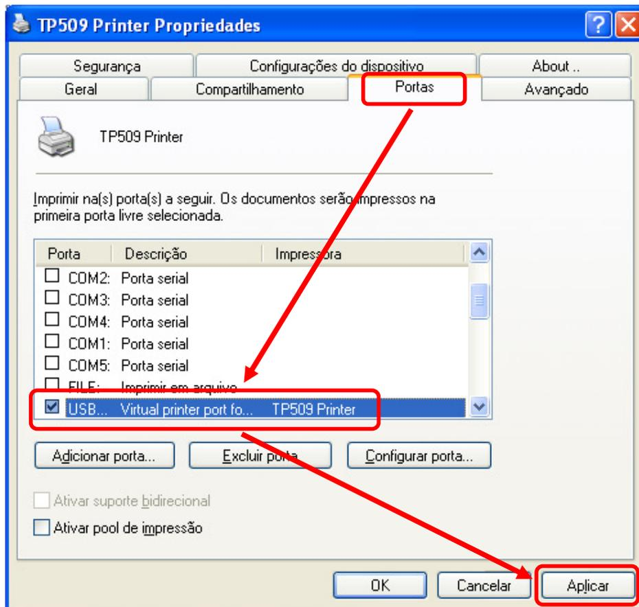
Choose the available USB port, such as the one shown in above and then click “Apply” to complete the configuration of USB port.
