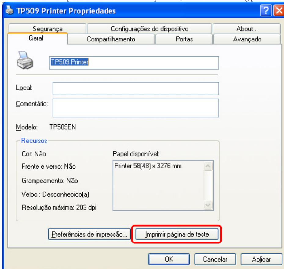
Click “Print Test Page” if the printer has connected to the computer and the configuration of communication port is correct, the printer would execute the print command , then print the test page.
